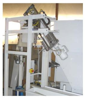
Drying at low temperature (on the average less than  $100^{\circ}$ C) on 6 drying positions.
