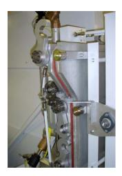
Automatic stripper of the belt type enabling to come out direct to a stacker with a capacity of 1,250 socks or a packaging machine
