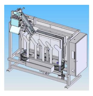
The machine is available with length control, a double stripper allowing to increase the productivity of the machine up to 600 pairs/h. In this case the machine will be fitted with 14 form legs.
